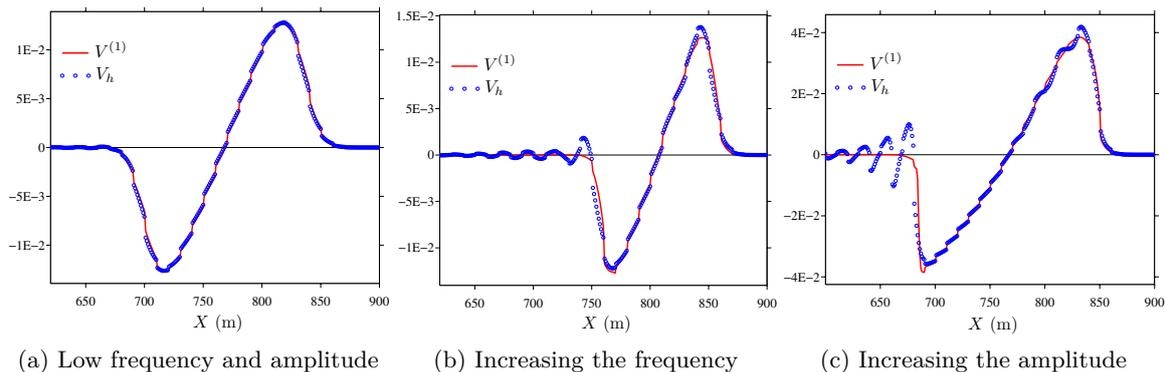
FIGURE 1 – Comparison of the velocity fields  $V_h$  and  $V^{(1)}$  obtained by full-field simulations and by first-order homogenization, respectively.
